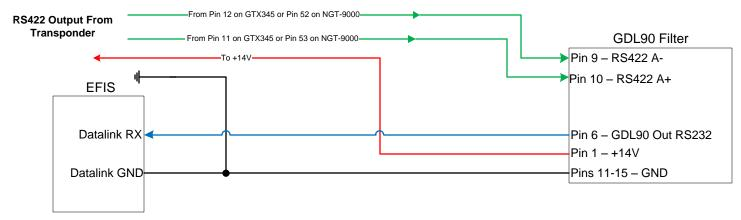
Install Note: GTX345 RS422 output needs to be set to OPT LGCY ADSB to provide weather and traffic to the GDL90 box. The only baud rate available is 115,200.
