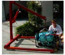
Figure 1. Engine Hoist
